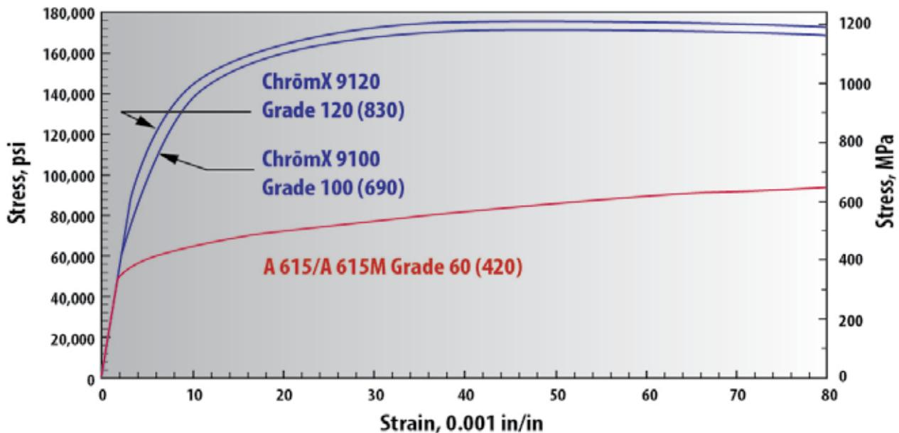
Tensile Properties of ChromX (ASTM A1035/A1035M) Reinforcing Bars
